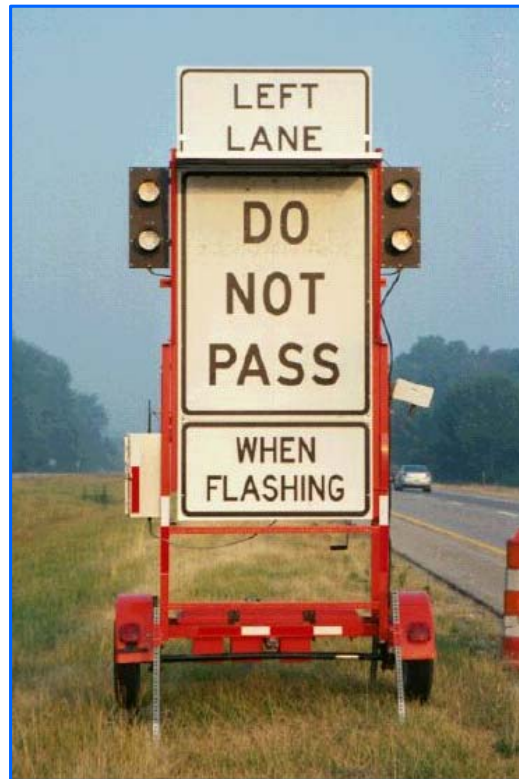
Figure 1: Dynamic Lane Merger Deployed On I-69 Near Lansing, Michigan
