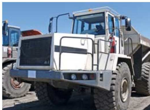
< Guardrails installed beside the engine bay of an articulated dump truck provide physical fall protection for pre-start checks and servicing.
