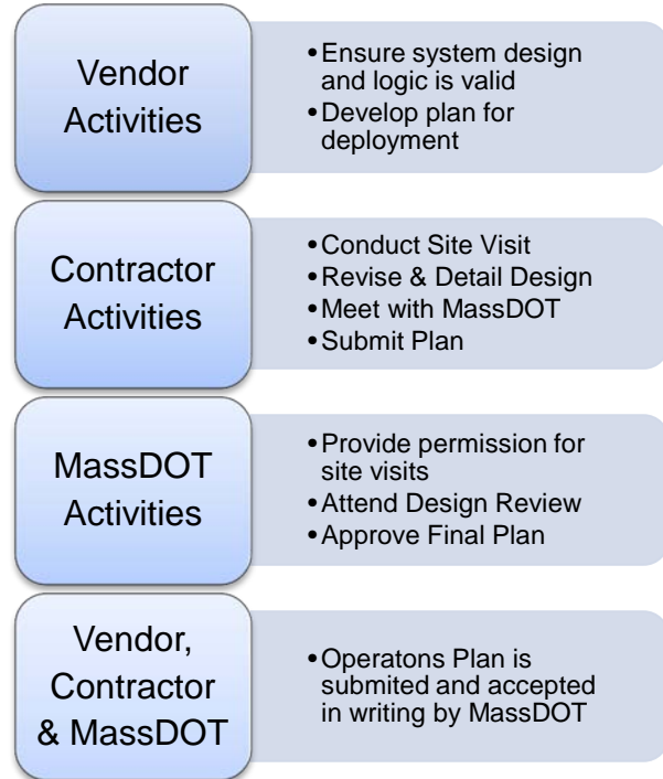
Figure 3: Preparation for Smart Work Zone Deployment
