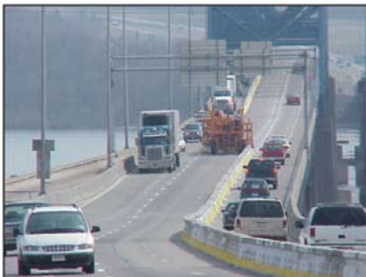
Figure 2. Moveable Concrete Barrier and Transport Machine
